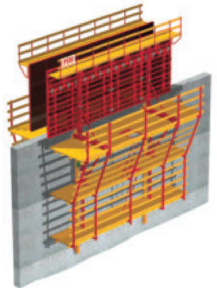
Example of the ACS R with additionally integrated working platforms, here for reinforcement work.
